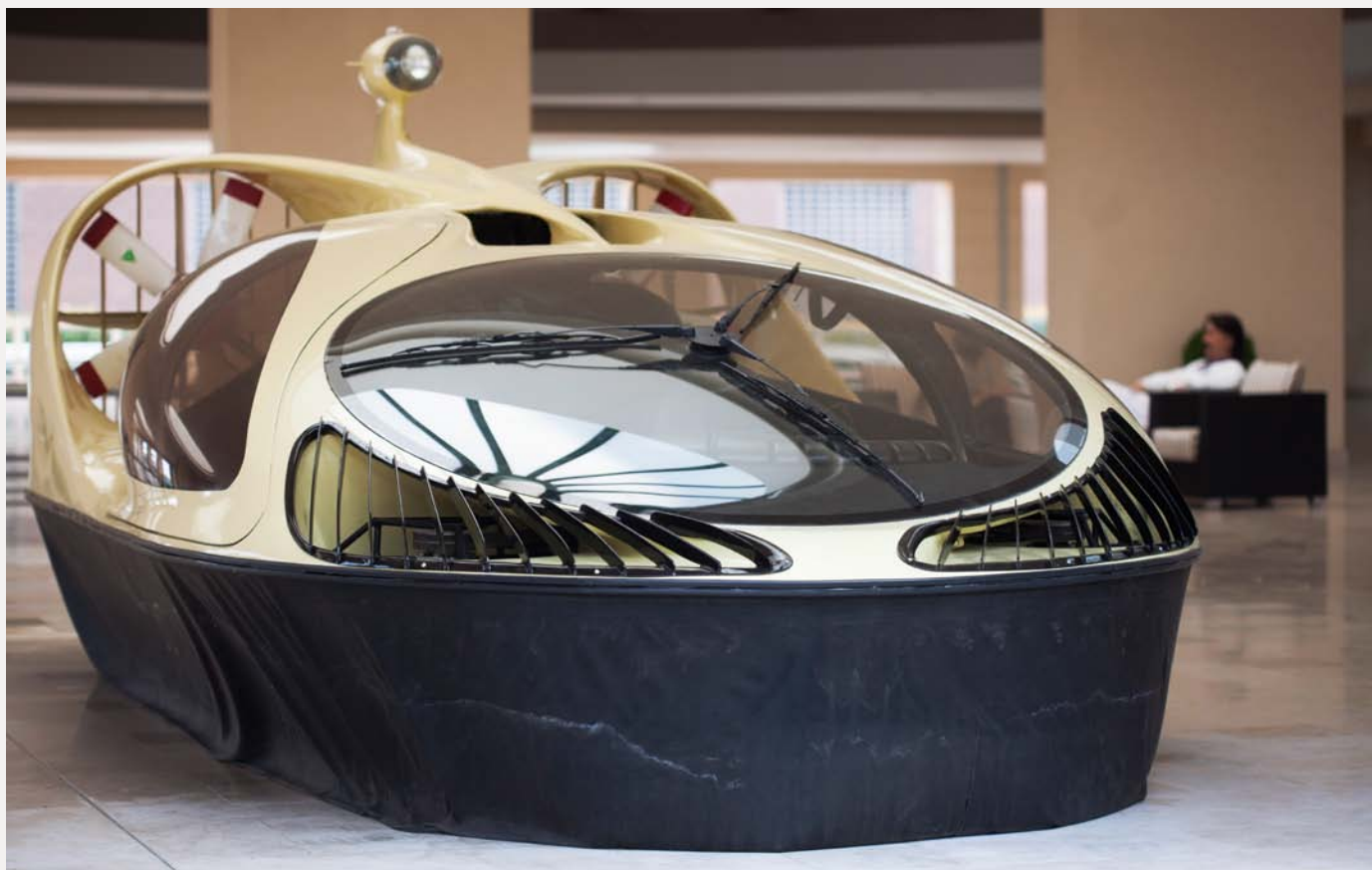
Fitted with a BMW engine, the Small Hovercraft (1998, mock-up) – a two- to four-seater AVC (air-cushion vehicle) – is designed to travel at speeds of up to 150 km/h.
